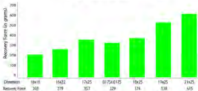
Peak force rated as archwires deflected 25mm over 1.0mm span
