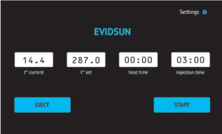
Heat-up timer stops at zero, and the injection timer will start the countdown. During the injection, heat is automatically turned off and the temperature drops.
