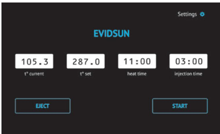
To change the set temperature, press its value, and the appropriate window will pop up. Permissible temperature range is from 0°C to 450°C. When temperature is set, press “Enter”.
